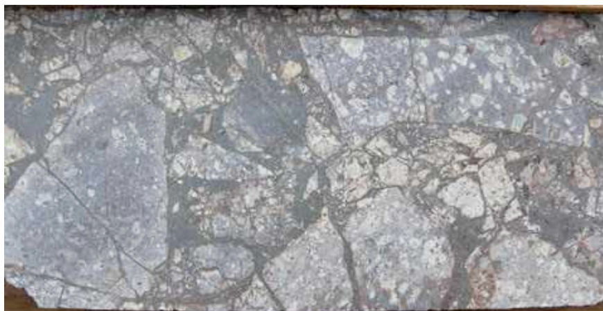
Figure 6. Less altered (grey to purple colored) igneous clasts in a specular hematite matrix. The clasts show sericitic alteration of feldspar phenocrysts (pale green color), but less obvious alteration of the volcanic groundmass, though the purplish color suggests weak hematization. Contrast the color of the clasts here with those in Figure 4. The clasts in this sample display apparently differing phenocryst abundance suggesting some movement during brecciation. There is a slight suggestion of bleaching on some clast rims. SJ-06-4, 131m.
