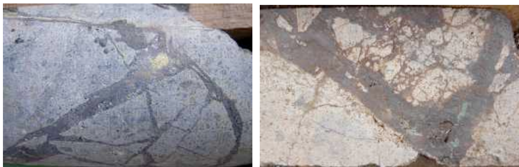
A. B. Figure 7. Typical copper mineralization at Cerro Verde. A. Weakly altered andesite-dacite cut by specular hematite vein with clot of chalcopyrite in vein center. SJ-06-7, 169m. B. Supergene oxidized version of A with green copper oxides in the center of a supergene weathered hematite vein. The location of the copper oxides suggests very little mobilization and migration of copper during the supergene event. SJ-06-4, 136m.
