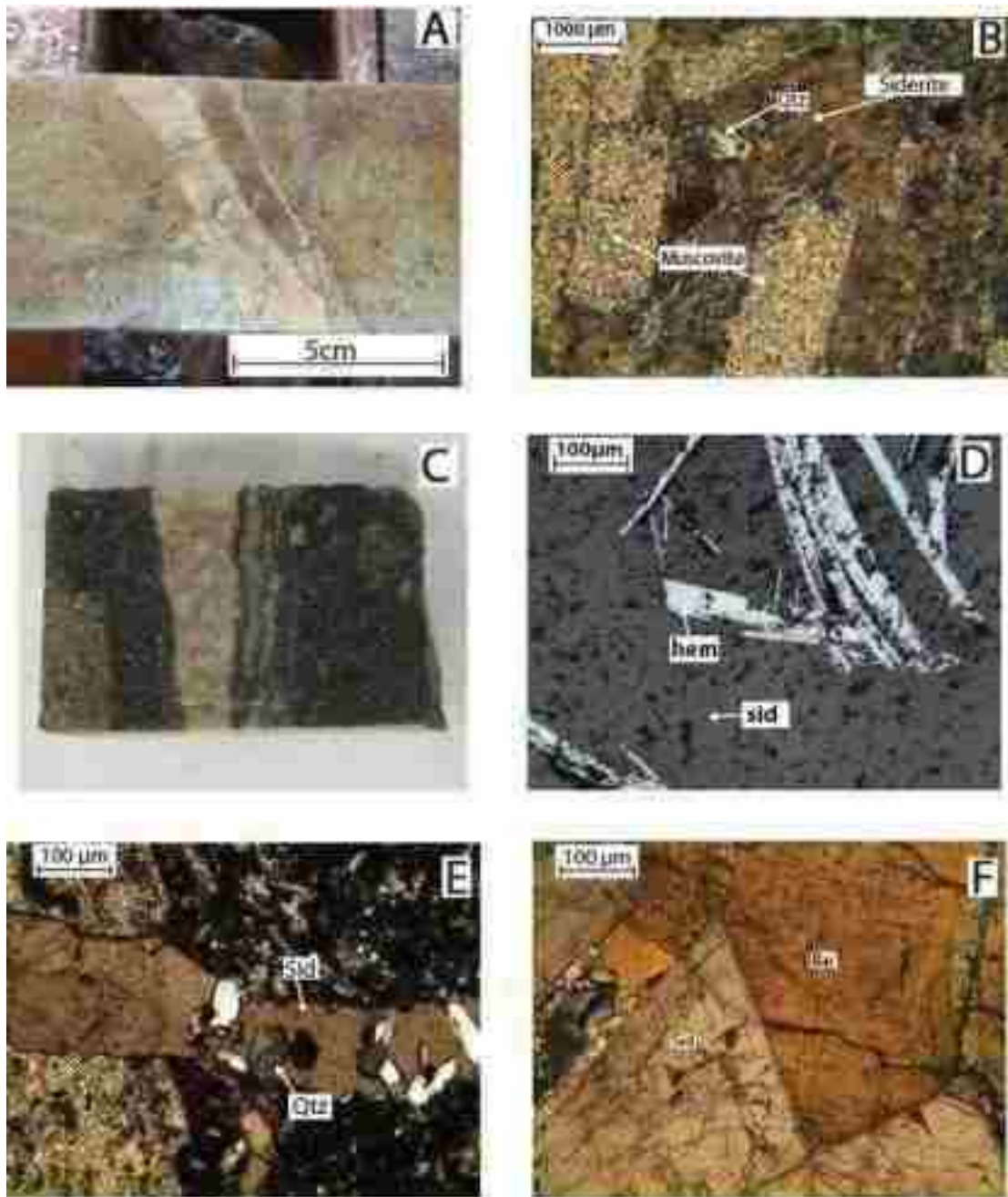
Figure 5.7 Siderite alteration and veining. A) Coarsely crystalline siderite vein surrounded by pervasive siderite altered host rock, SJ-06-01. B) Photomicrograph of siderite alteration. Masses of fine-grained siderite overprinted earlier muscovite alteration, SJ-07-62 38m. C) Alternating bands of hematite and siderite, SJ-07-17 83m. D) Photomicrograph of siderite replacing hematite, siderite fills in ragged dissolution textures on the hematite crystals, SJ-06-25 123m. E) Euhedral quartz grains encased in a siderite vein, SJ-06-37 108m. F) Coarse-grained siderite cut and surrounded by barite, SJ-06-24 111m.
