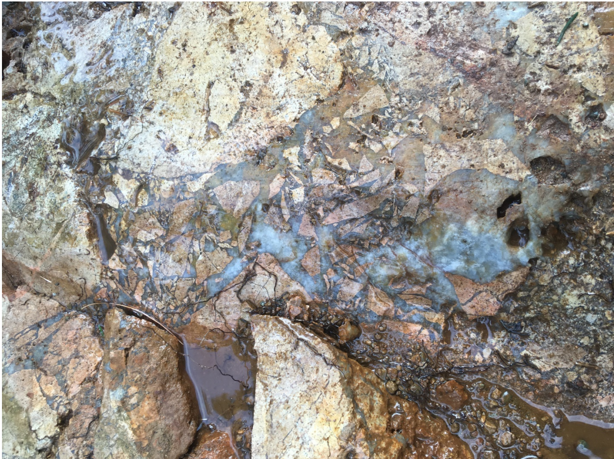
Figure 9-7: Trench 1 example of brecciated albitite with quartz-carbonate-pyrite matrix.
